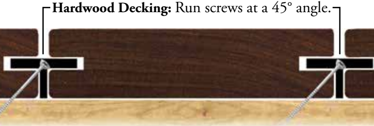
Shown Above: Ipe (Brazilian Walnut) Hardwood decking installed with DeckWise® Extreme™ hidden deck fasteners.
